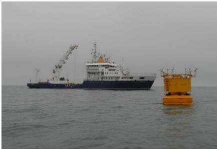
*Deployment vessel and the FLiDAR on site*
