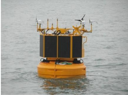
*The FLiDAR buoy deployed in the Irish Sea, UK*
